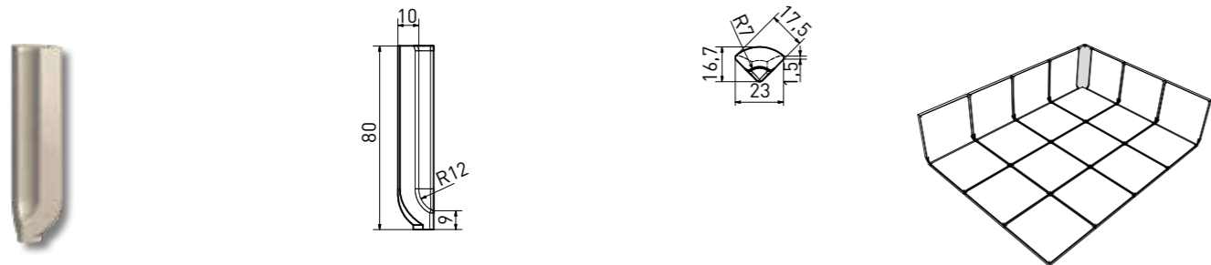
inside corner skirting plinth | TSIRH... | 80×23×10 mm
