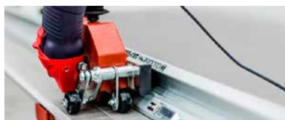
Fig. 7 - A cutter with a guide bar and clamping suction
