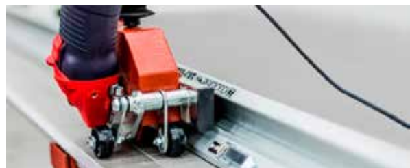
Fig. 7 – A cutter with a guide bar and clamping suction
