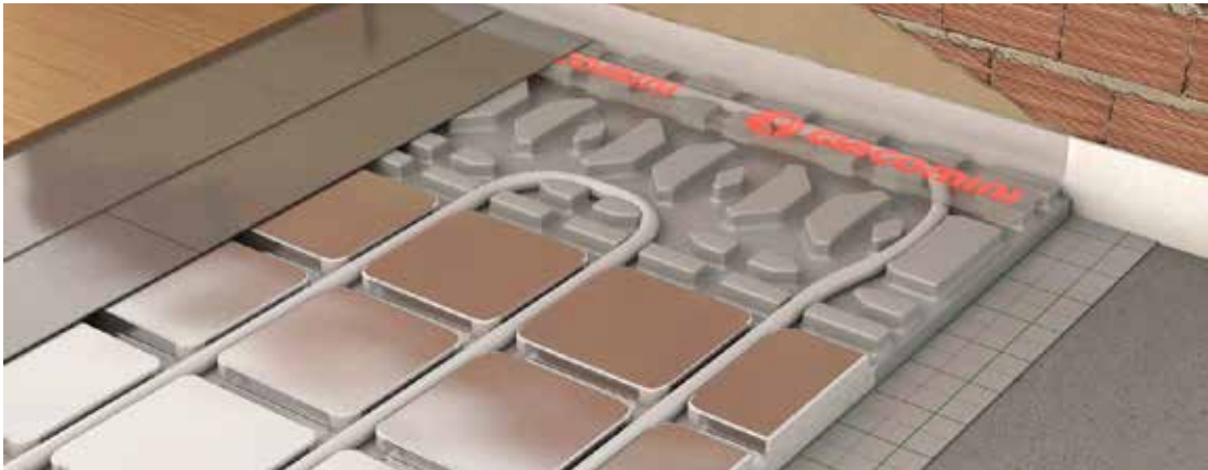
Fig.19 Dry system of thin-layer water-based underfloor heating
